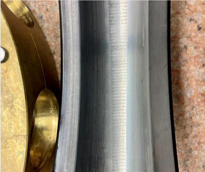
Figure 12. Bearing C4 outer ring with Current Leakage damage
