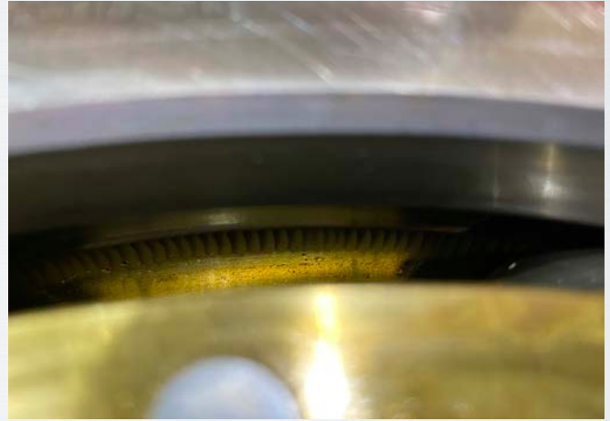
Figure 16. Bearing I8 with Electrical Erosion damage
