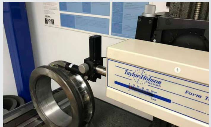
Figure 10. Inner ring surface quality inspection of the received bearings.
