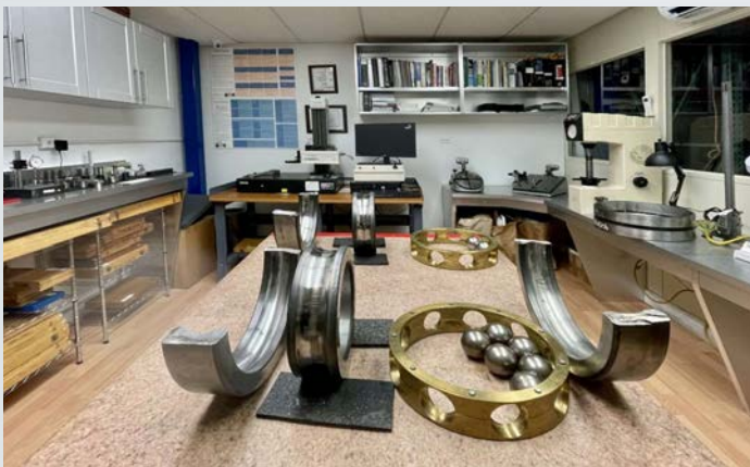
Figure 9. Disassembled bearings ready for inspection at ABS facility.
