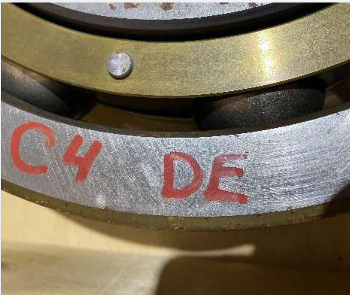
Figure 14-1. Bearing C4 with Electrical Erosion
