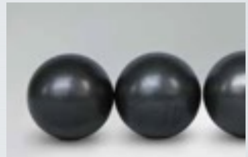
Figure 3. Electrical corrosion has a dark color that covers the entire ball surface [8]
