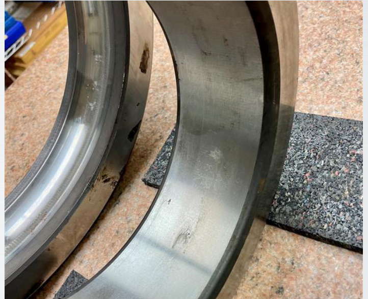
Figure 13. Bearing C4 with Current Leakage and Excessive Voltage cratering damage
