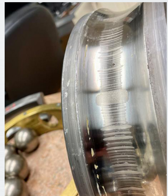
Figure 11. Bearing C4 inner ring with Current Leakage damage
